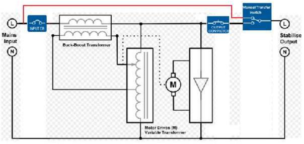
MRG/MSR33 Series Servo Voltage Regulator Boundary Diagram
